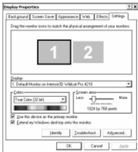
Figure 14. Dual Monitor Settings Tab
