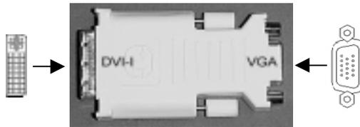
Figure 4. DVI-I to VGA Adapter
