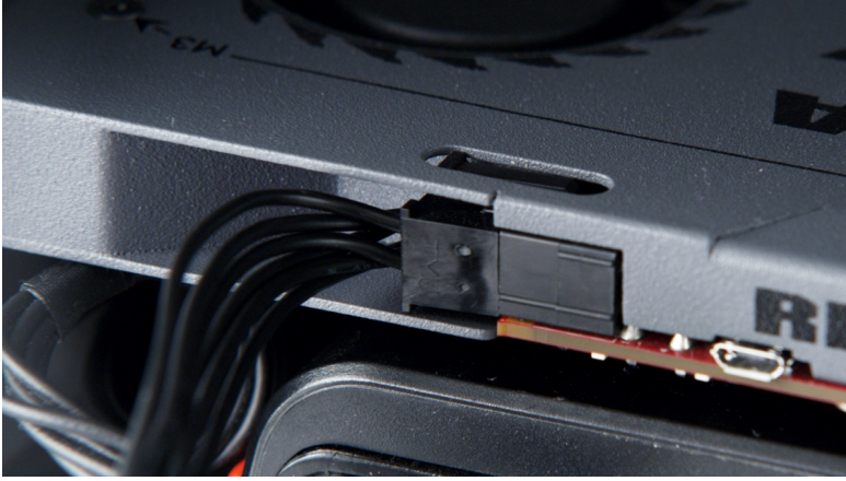
Figure: Connect Power to RED ROCKET-X
