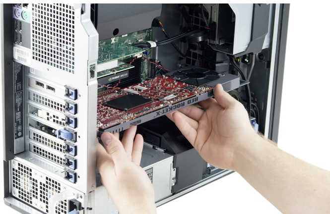
Figure: Insert RED ROCKET-X
