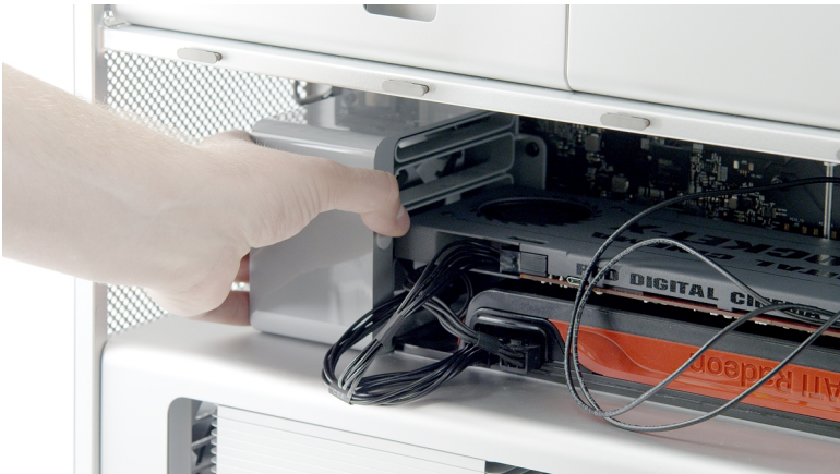
Figure: Slide PCIe Fan to Original Position
