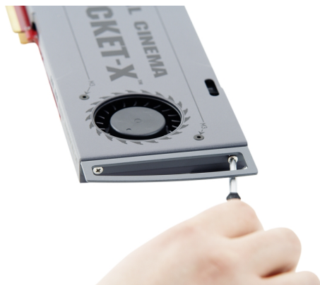
Figure: Attach PC Extender
