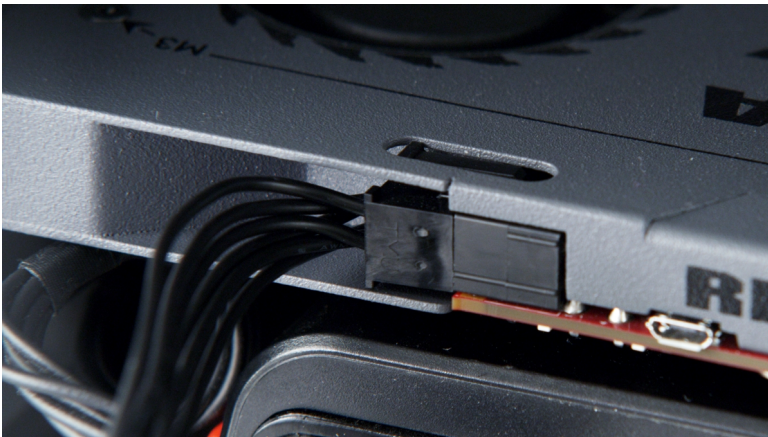
Figure: Connect Power to RED ROCKET-X
