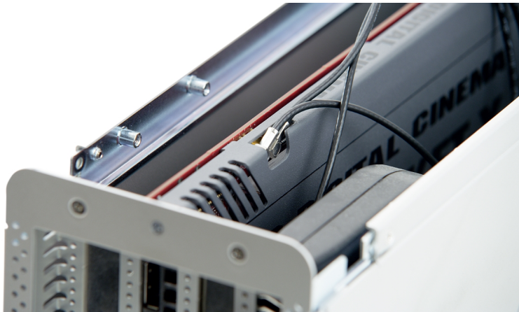
Figure: Connect HD-SDI Slot Filler to RED ROCKET-X
