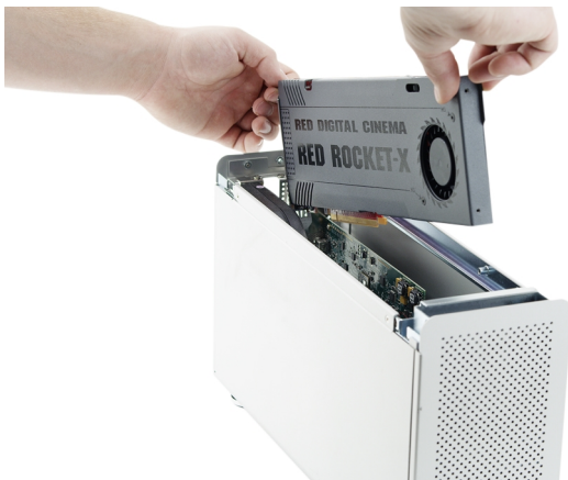
Figure: Insert RED ROCKET-X
