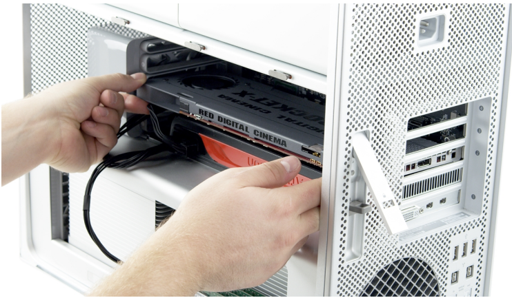
Figure: Insert RED ROCKET-X
