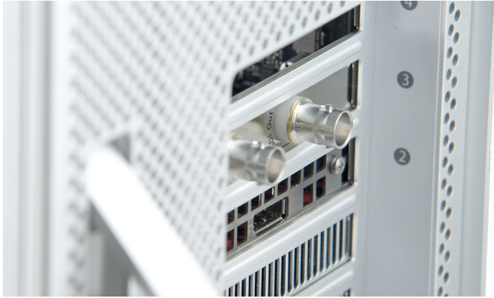
Figure: Install HD-SDI Slot Filler
