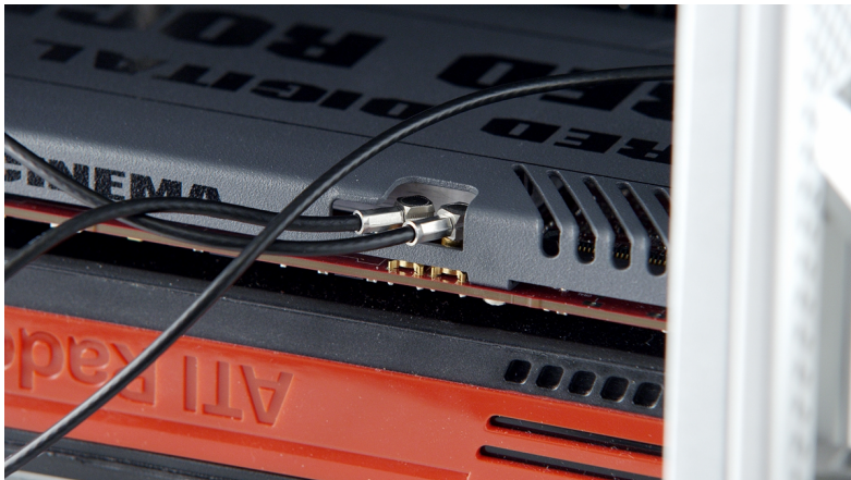
Figure: Connect HD-SDI Slot Filler to RED ROCKET-X
