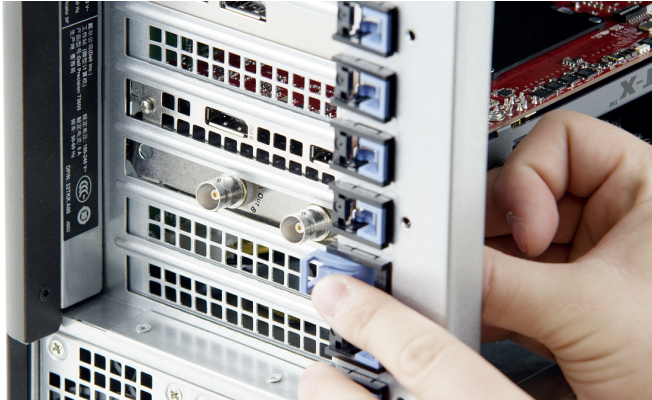
Figure: Install HD-SDI Slot Filler
