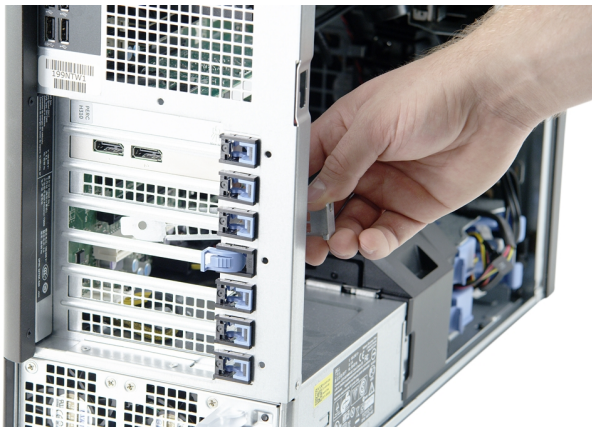
Figure: Remove Slot Bracket
