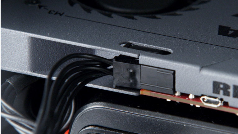
Figure: Connect Power to RED ROCKET-X
